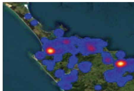
Figure 8-3: Geographical Distribution of At-Risk Isolating Equipment Across Different Extreme Weather Conditions
