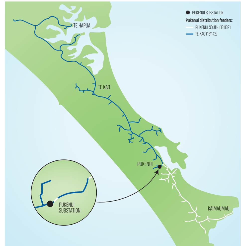
Figure 3-3: Geographic Diagram of the Pukenui Zone Substation
