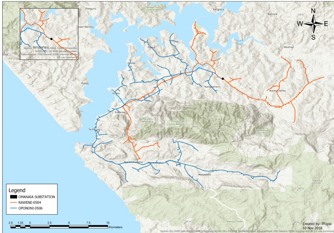
Figure 3.13: Geographic diagram of the Omanaia zone substation
