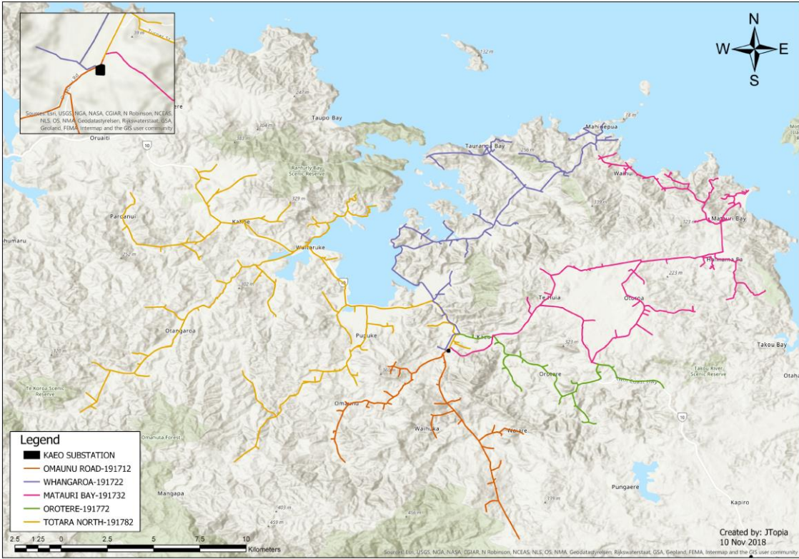
Figure 3.9: Geographic Diagram of the Kaeo Substation
