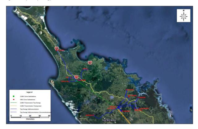
The network receives supply from the national grid at the Kaikohe substation and from local generation at Ngawha. The Kaikohe substation supplies the southern part of the network directly, with the northern part of the network supplied from a single transmission circuit to Kaitaia. Electricity is then distributed to consumers across long distribution feeders supplied from a limited number of zone substations.
