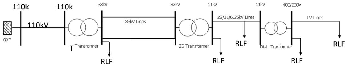
Figure 1: RLF Application at Different Network Stages
